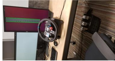
Fig. 4: The system (rotated 90 degrees) used for collecting driving performance data from human testers: A logitech driving wheel, acceleration and braking paddles, and a chair.
